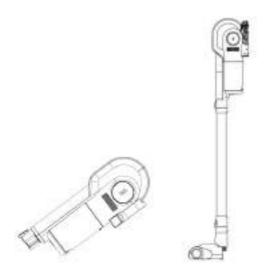
2, Mount the suction pipe and floor nozzle on the motor unit.
