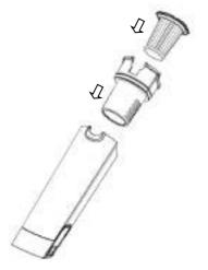
6, Put the dust cup into the machine.
